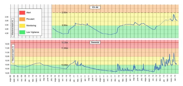
Figure 5. Groundwater levels at Danestal since august 2009 and A4 since august 2010 and critical water level for warning system
