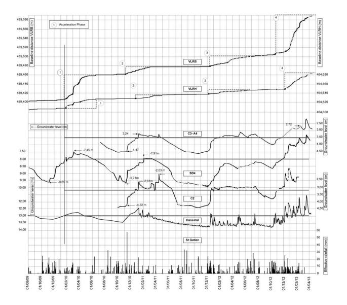
Figure 4. Relations between the displacements (GNSS VLRH and VLRB), piezometric levels (SD4 and C2), pore pressure (A4) recorded at Cirque Graves and daily rainfall of St Gatien station
