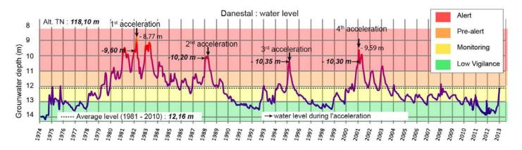
Figure 3. Groundwater level at Danestal since 1974 and critical water level for warning system
